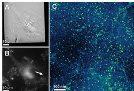
The electron microscopy images were correlated with their corresponding location in the light microscopy image. The rectangular design of the E-chip window served as a reference system for matching position coordinates between images.
