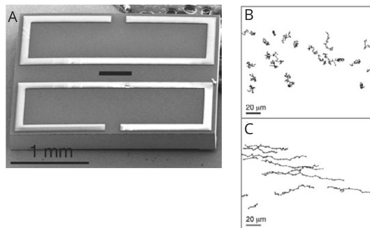
An SEM image of the GapSet E-chip used to form the channel is shown in Figure A. Under static liquid conditions, the trajectories of the polystyrene microspheres
