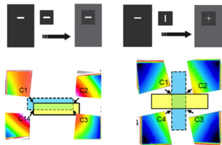
**Figure 3:** The top figure shows the parallel (left) and crossed (right) window configurations. The bottom left figure illustrates how a slightly misaligned windows in the parallel configuration leads to thick liquid layers. The bottom right figure illustrates window bowing in the crossed configuration. In this configuration the corners always provide the thinnest liquid layers. The designations C1-C4 refer liquid thickness maps taken at each of the four corners of the window.
