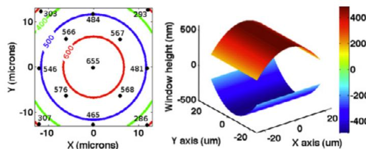
**Figure 4:** The left figure shows a thickness map measured using EELS. The right image is a simulation showing the effects of window bowing in the crossed configuration.
