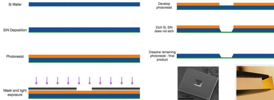
**Figure 1:** Poseidon E-chip fabrication. Starting with a silicon wafer, a silicon nitride membrane is deposited. A layer of photoresist is deposited then exposed to UV light through a photomask. The exposed photoresist is dissolved leaving a small silicon window. The wafer is immersed in an etchant that preferentially dissolves silicon leaving a thin SiN layer. An SEM image and photograph of completed E-chips are shown in the bottom right.
