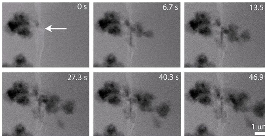
**Figure 1:** Series of ADF STEM images showing nucleation and growth of Li metal from GC electrode.
