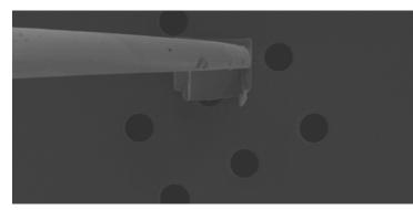
**Figure 4.** Lamella in contact with the heating membrane of the E-chip.
