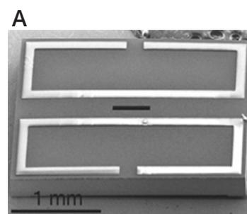
An SEM image of the GapSet E-chip used to form the microfluidic channel is shown in Figure A. Figure B shows a STEM image of nanoparticle flow. A series of streaks is visible at arrow 1, which presumably are due to a single gold nanoparticle moving to the left.
