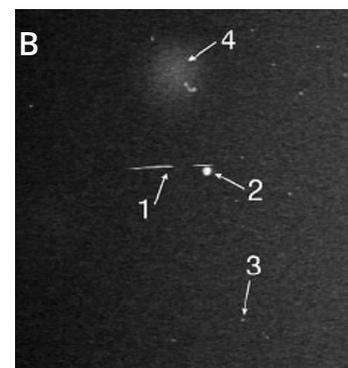
Arrow 2 highlights a stationary 100 nm gold nanoparticle, which was deposited on the silicon nitride window during flow. Several 30 nm diameter gold nanoparticles, such as that seen at arrow 3, are visible throughout the image.
